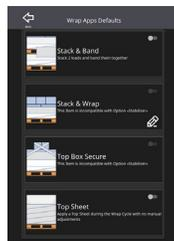
Eliminates the need for operators to make machine adjustments for common load requirements (e.g. stack & band, stack & wrap, labels, cornerboards, top sheet, top box, short loads)
